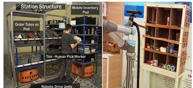
Figure 1: Left image shows Kiva systems carrying rack to human for picking objects 1 . Right image shows the robot manipulator system used for picking objects.
